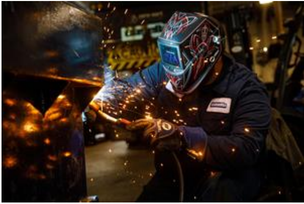
A Casella diesel technician uses a welder to repair a container.
